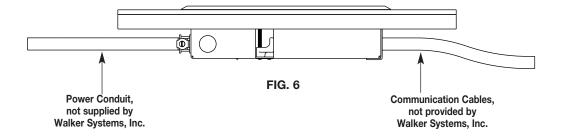
NOTE: The communication conduit plate does not need to be attached behind a compartment used for low voltage. Where required by local codes, connect conduit to the communication conduit plate. Type CMP communications plenum cable is required in raised floor plenums when wiring methods as described in NEC Article 300-22 are not followed.
