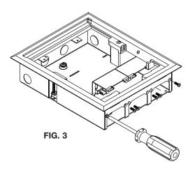
**Step 3** Place Walker Shallow Raised Floor Box in opening created in step one. (See Fig. 4.)
