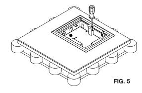
Step 5 Remove appropriate knockout(s) and feed flexible conduit to the floor box. Pull wires into the box and connect conduit to the box with a conduit connector. Pull communication wires into box. (See Fig. 6.)
