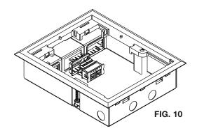
Step 10 When the box is not in service, the wire retainer should be installed (textured side up) to block off the cable exit. (See Fig. 11.) Otherwise, any exiting cables should be routed through the wire retainer prior to closing the lid. (See Fig. 12.)
