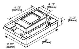
Fire Classified Two-Compartment Box – For use in either concrete or wood floors. Fully adjustable with tunnel compartment. Supplied with one (1) duplex receptacle, mounting plate, and one (1) communication mounting plate (RFB22AB). Other device plates sold separately.
