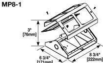
Same as MP8, except mounts on PK and N-R-G Presets, one No. 2, or one No. 4 duct. On Walkerduct Pro Series the fitting can be installed on any two-duct system. Overall capacity is 104.3 cu. in. [1709 cu cm]. Has 1/2" and 3/4" trade size concentric knockouts on each end. Fitting also provides one 1" trade size knockout in baseplate.
