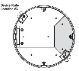
NOTE: Standard sizes for device plates for Plate Location 3 are 5 7/32" [132mm] x 2 3/4" [62mm].
