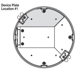
NOTE: Standard sizes for device plates for Plate Location 1 are 6 11/32" [161mm] x 2 3/4" [62mm].
