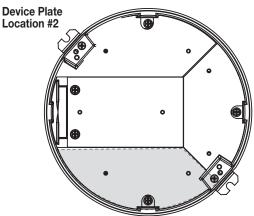
NOTE: Standard sizes for device plates for Plate Location 2 are 5 7/32" [132mm] x 2 3/4" [62mm].
