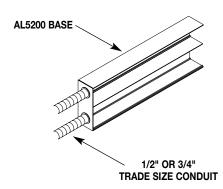
**End feeding:** AL5210B2/AL5210B3 and AL5210B3 Series end fittings have concentric 1/2" and 3/4" trade size KOs in end. Provide Electrical feed through KOs. Insert fitting into End of raceway base. Secure in place by tightening two screws.
