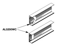
For retaining wires in long raceway run, Snap-in AL5200WC Series Wire Clips into AL5200B Base as required.
