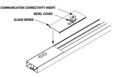
**To Install:** Snap-in Bezel Cover into AL5256 Device place. After installing the bezel, Snap-in the communication connectivity into the bezel cover as required. Snap-in AL5656 Device Place Series into AL5200B Raceway base to complete install.
