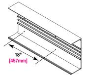
To attach AL5200B Series Base sections to mounting surface, drill 9/32" holes in The base (approx. 18" O.C.) Fasten with #8 flat head screws.
