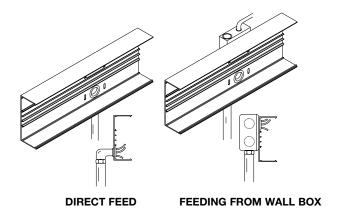
AL5214 Wall Box Connector connects to two in line AL5200B base sections via AL5201 Couplings supplied.
