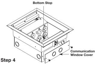
Place device plate in box. Position bottom of plate behind stops in floor of box. Roll plate into position and mount with screws provided.
