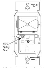
Adjustment controls are located behind the front cover of the unit and are clearly labeled.
