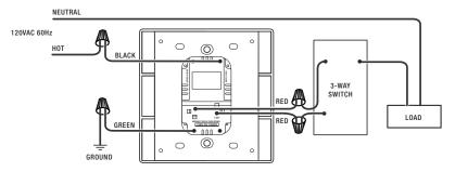
Fig. 6: Multi-way Wiring
