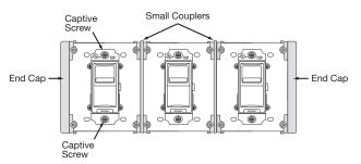
Fig. 11: Install Dimmers and Attach Small Couplers
