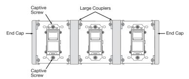
Fig.9: Install Dimmers and Attach Couplers
