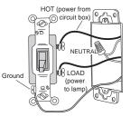
Fig 2: Typical Single Pole Switch Wiring
