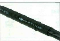
T&B's heat shrinkable tubing is made of thermally stabilized cross-linked polyolefin. This provides a recovered wall thickness greater than that of the cable jacket replaced. The insulating covers which have an internally applied sealant offer protection against moisture, may be used over lead, steel, aluminum, copper, standard plastic and elastomeric insulating materials.
