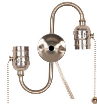
80-1269 Satin Nickel Twin Pull Chain Satin Nickel Chain and End Ball with 14" 18/2 SPT-2 105°C Clear Silver Wire 7" Centers 1/8 IP Top and 1/8 IP Bottom 660W-250V
