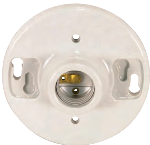
90-445 2 Terminal 80-1648 4 Terminal Keyless Glazed Porcelain Ceiling Receptacle Screw Terminals 660W-250V
