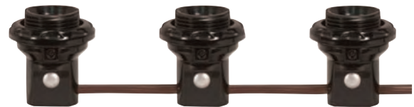
80-1474 1 1/4" with Shoulder and Phenolic Ring 6" Centers 18" Tail 18/2 SPT-1 105°C Brown 75W-125V
