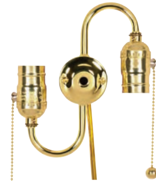
80-1268 Brite Gilt Twin Pull Chain Brite Gilt Chain and End Ball with 14" 18/2 SPT-2 105°C Clear Gold Wire Internal Wire-18 AWM 105°C 7" Centers 1/8 IP Top and 1/8 IP Bottom 660W-250V
