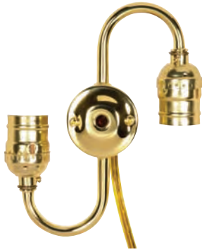
80-1189 Brite Gilt Twin Keyless with 14" 18/2 SPT-2 105°C Clear Gold Wire Internal Wire-18 AWM 105°C 7" Centers 1/8 IP Top and 1/8 IP Bottom 660W-250V
