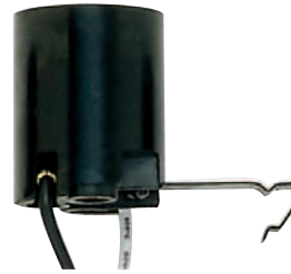
90-543 Snap-In Socket for 6" Pans Bracket Extends 1" from End of Socket 8" AWM B/W Leads 105°C 660W-250V
