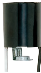
90-1151 10" AWM B/W Leads 105°C 1/8 IP Hickey 660W-250V
