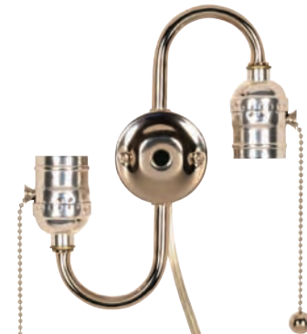
80-1270 Nickel Twin Pull Chain Nickel Chain and End Ball with 14" 18/2 SPT-2 105°C Clear Silver Wire Internal Wire-18 AWM 105°C 7" Centers 1/8 IP Top and 1/8 IP Bottom 660W-250V
