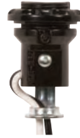
90-1557 1 1/4" w/Shoulder and Phenolic Ring 8" AWM B/W Leads 105°C Pulled Thru 1/8 IP Inside Extrusion 75W-125V
