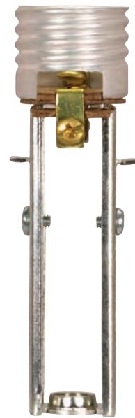
90-404 4" to 5 1/2" Keyless - 1/8IP Screw Terminals with Paper Liner 660W-250V
