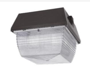
Medium size ceiling mount fixture: 26, 32 and 42 Watt compact fluorescent available. Housing is die cast aluminum with clear vandalproof polycarbonate refractor. Photocontrol, Sensor (CFL 120v only) models available. Lamp supplied.
