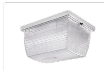
Compact ceiling mount fixture: 7, 9, 13, or 14 Watt fluorescent. Reflector is dieformed heavy gauge steel in white finish with clear vandalproof polycarbonate refractor. Lamp supplied.
