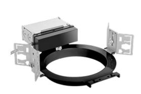
Easy to install 4" and 6" rough-in with die-cast aperture ring, removable driver, thermal protector and adjustable butterfly brackets. This rough-in is designed to make new construction recessed downlighting easy Available with 80 or
