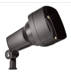
Rugged die cast floodlight with heavy mounting arm, lens, glare shield and weatherproof silicone gasket. 75 Watt max., accepts lamp types PAR16, PAR20 and R type. 120 volt Lamp not supplied.
