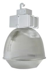
Indoor fixtures for use below 25'. 16" units for 250w Metal Halide. 22" units for 400w Metal Halide. Die cast aluminum housing and wiring box. Clear acrylic Lexalite Reflexor prismatic refractor. Ballast and lamp supplied.
