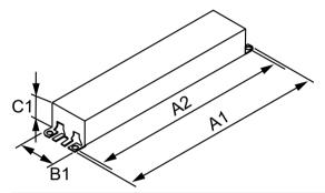
ELE DIMMING BALLAST (3) F32T8 120-277V
