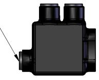
**WIRE ENTRY PORT** WIRE RANGE: 750KCMIL - 250 PRE-FILLED W/ OXIDE INHIBITOR
