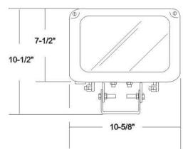
Yoke Rotation Capability: Side to side rotation aiming = none. Up tilt aiming from horizontal = 45° max (the yoke allows for straight up aiming but this could allow for water build up so 45° is what we should go with. Down tilt aiming from horizontal = 45° max (the yoke allows for straight down aiming but this could allow for water build up. Uses weep holes.
