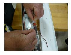
6. CLOSE FIXTURE AND REINSTALL SCREWS FROM STEP #1 (ENGAGE ONE SIDE AND APPLY MINIMUM PRESSURE ON OPPOSITE SIDE TO CLOSE LUMINIARE)
