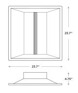
NOTE: Use of Expanded Junction Box will expand the depth to  $6.67^{\prime\prime}$  and Emergency Backup will expand the depth to  $6.30^{\prime\prime}$ .
