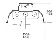
**A**= 1/4 x 1/2 (.635 x 1.27) hole C = 7/8 (2.22) dia. K.O.**D**= 11/16 (1.75) dia. K.O.
