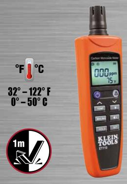
The **ET110** is an easy-to-use meter that detects and measures concentration levels of carbon monoxide (ppm) and temperature (°F/°C). Backlit LCD screen for easy viewing in low light; warning indicator light blinks green for clean and red for CO detection.
