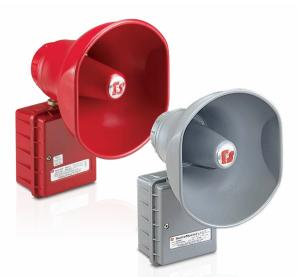
The AM300 and AM302 are rugged, transformer coupled, re-entrant speakers for use in public address or paging applications. These 15 and 30 watt speakers feature a durable speaker cone and projector constructed of spun aluminum. The speaker wiring connections are enclosed in a dust- and moisture-proof, die-cast aluminum compartment. All external surfaces are sealed with a red or gray powder coat paint.
