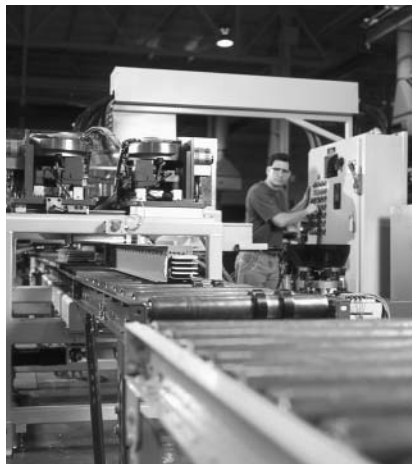
Final Busway Assembly
