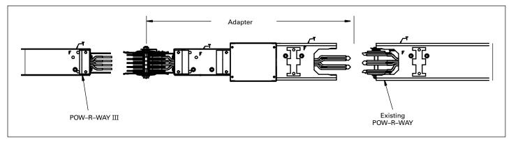
Figure 48. Pow-R-Way III to Pow-R-Way adapter
