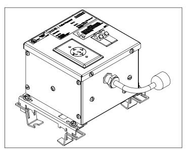
Figure 72. Single receptacle plug
