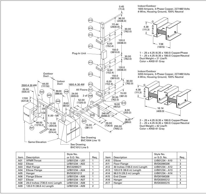
Figure 79. Sample installation drawing
