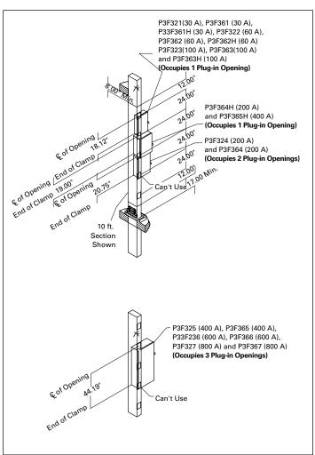
Figure 61. Fusible plug-in device mounting
