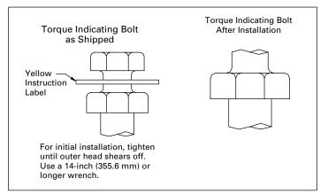
Figure 82. Torque indicating bolt
