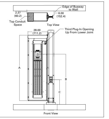
Figure 46. Busway-connected panelboard detail
