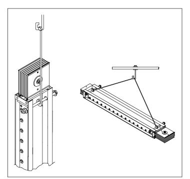
Figure 80. Hoisting riser and horizontal busway
