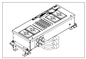
Figure 73. Quad receptacle plug
