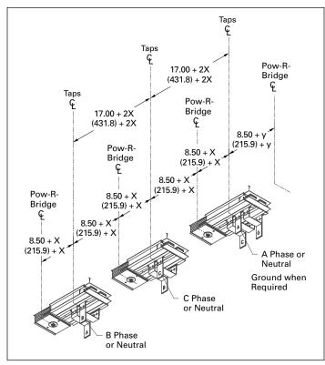
Figure 33. Three single-phase transformer taps
