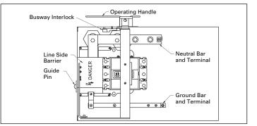
Figure 74. Typical circuit breaker plug-in unit
