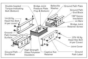
Figure 7. Indoor bridge joint features
