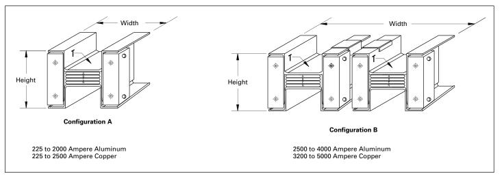
Figure 14. Pow-R-Way III cross-section dimensions
