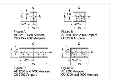
Figure 9. Pow-R-Bridge joint
