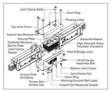
Figure 8. Outdoor bridge joint features
