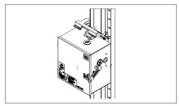
Figure 75. Vertically mounted plug
