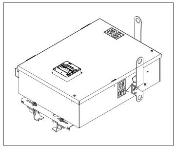
Figure 63. Surge protective device (SPD Series) bus plug
