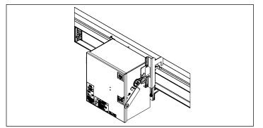
Figure 76. Horizontally mounted plug
