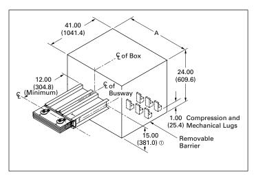
Figure 29. Weatherhead details
