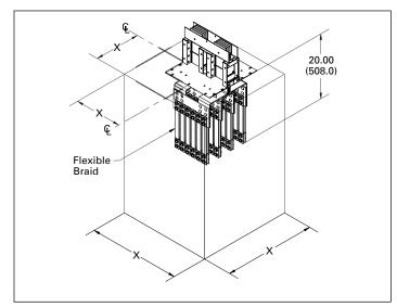
Figure 37. Transformer flange connections
