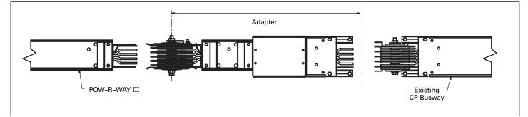
Figure 49. Pow-R-Way III to CP adapter
