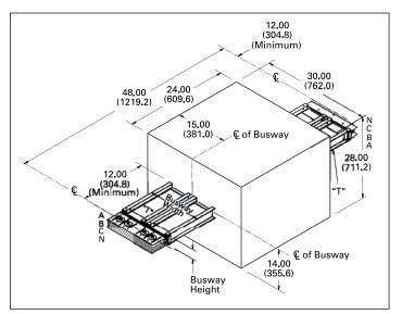
Figure 31. 180° transposition – dimensions in inches (mm)
