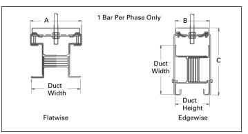
Figure 53. Hook hangers-non-seismic only
