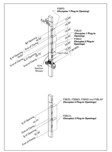
Figure 62. Breaker plug-in device mounting
