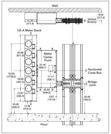
Figure 41. Bridge joint PTO
