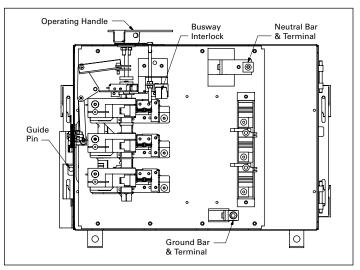
Figure 77. Typical fusible plug-in unit
