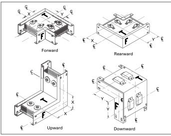
Figure 18. Corner joint elbows (for indoor applications only)
