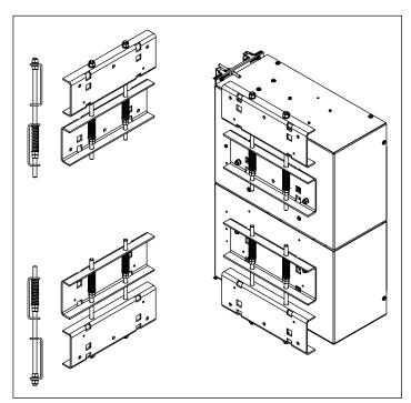
Figure 47. Panelboard spring hangers
