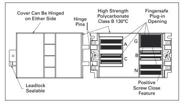
Figure 12. Plug-in outlet cover
