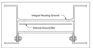
Figure 13. Housing ground vs. internal ground
