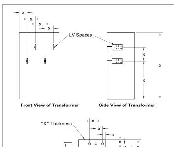
Transformer Tank Wall LV Spade Detail
