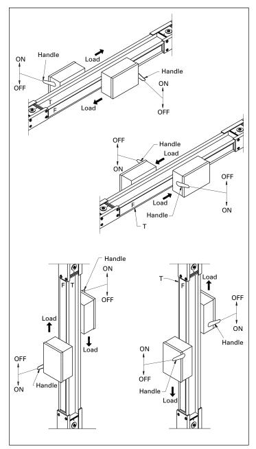
Figure 60. Plug-in device mounting
