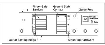
Figure 59. Plug-in outlet details
