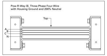
Figure 4. 200% Neutral cross section
