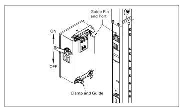
Figure 58. Plug-in stab details
