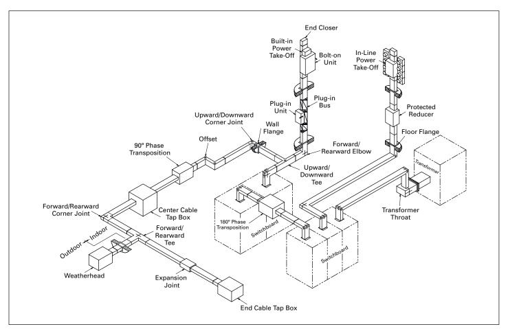
Figure 16. "T" and "F" orientation for fittings
