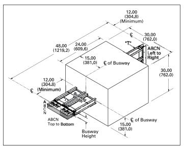
Figure 32. 90° transposition-dimensions in inches (mm)
