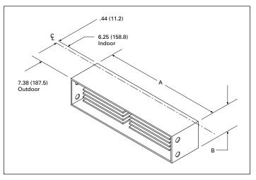
Figure 52. End closure with Pow-R-Bridge removed
