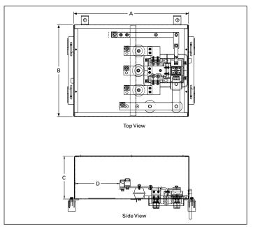
Figure 71. Plug-in cable tap box
