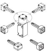
Actuator can be repositioned for horizontal or vertical installation. The operating heads can be rotated manually in 90° steps to suit the specified direction of operation. LS-...ZBZ
