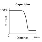
The **output circuit** remains active until the target leaves the sensing field. The oscillator responds with a decrease in amplitude, and when it is no longer receiving sufficient capacitance feedback, the detector circuit switches OFF.
