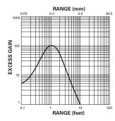
**Note:** The excess gain charts in this catalog represent the minimum excess gain provided by the sensor (unless otherwise noted). Actual performance may be better.
