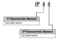
An enclosure with this designation is protected against the penetration of solid objects greater than 1.0 mm and against splashing water.
