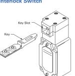
Actuation of the interlock switch occurs only when the corresponding key is inserted into the key slot. The key is usually mounted on a door or machine guard in such a way that when the door or the guard is closed, the key fits into the slot actuating the switch. The special key design makes the safety interlock switch extremely difficult to defeat. When inserted into the slot, the key performs three separate mechanical functions.
