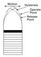
With hysteresis, the operate point and the release point are slightly different distances from the sensor face
