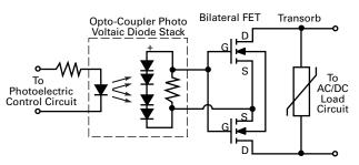
develop the fixed voltage drop across its terminals like other solid-state switches. It also does not require any residual or leakage current to keep the electronics powered in the OFF-state.
