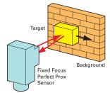
Perfect Prox is a special type of diffuse reflective sensor that combines extremely high sensing power (excess gain) with a sharp optical cutoff. This allows the sensor to reliably detect targets regardless of variations in color, reflectance, contrast or surface shape, while ignoring background objects that are just slightly beyond the target range. See **Page V8-T12-28**.
