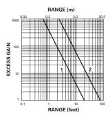
1. 12100A and 12100R detectors using 11100A or 11100R sources 2. 12102A detectors using 11102A sources
