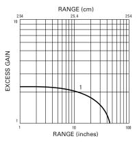
Clear object detector 3 in retroreflector 1. 1452E
