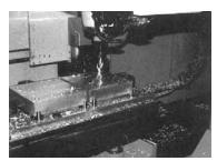
An Inductive Proximity Sensor Monitors Drilling Operation
