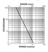
Gain using E51KF823 fibers 1. 13150A Prism
