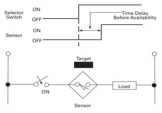
Once the target enters the sensing range and the detector causes the output to change state, a certain amount of time elapses. This is called **response time**. For an AC sensor this is usually less than 10 milliseconds. DC devices respond in 1 millisecond or less.
