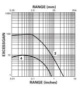
Gain using E51KF723 fibers, based on 90% reflective white card 3. 13100A Comet
