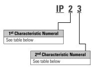
An enclosure with this designation is protected against the penetration of solid objects greater than 12 mm and against rain.
