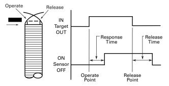
Similarly, when the target leaves the sensing field there is a slight delay before the switch is restored to the OFF state. This is referred to as the **release time**. An AC sensor typically releases in one cycle (16.66 milliseconds) and DC devices usually in 1 millisecond, or less.
