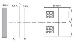
A = Rated Sensing Range B = Maximum Usable Sensing Range C = Maximum Reset / Release Range
