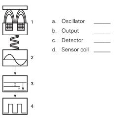
Match the proximity sensor component with its function.
