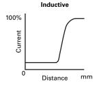
The **detector circuit** monitors the oscillator's output. When it detects sufficient change in the field, it switches on the output circuit.
