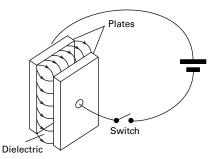
When this principle is applied to the capacitive proximity sensor, **one capacitive plate is part of the switch, the enclosure (the sensor face) is the insulator. The target is the other "plate."** Ground is the common path. Capacitive proximity sensors can detect any target that has a dielectric constant greater than air. Liquids have high dielectric constants. Metal also makes a good target.
