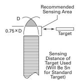
On a slide-by, or **lateral approach**, the target approaches the center axis of the sensing field from the side. The target should not pass closer than the basic tolerance built into the machine design. Targets bumping into your sensor are a sure guarantee of eventual poor sensor performance.
