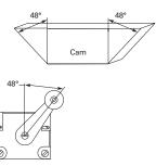
When using side-push or toppush plunger actuators, be sure the cam operates in line with the push rod axis. **Do not use the limit switch body to act as a mechanical stop for the cam in overtravel applications.** Some other type of barrier must be provided as the stop. 171
