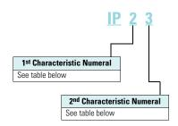
An enclosure with this designation is protected against the penetration of solid objects greater than 1.2 mm and against rain.
