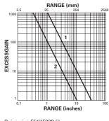
Gain using E51KF823 fibers 1. 13100Å Comet 2. 13106A Comet
