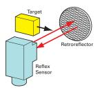
The source and detector are mounted in a single sensor housing and are positioned parallel to one another on the same side of the object to be detected. The light beam is transmitted from the source to a retroreflector that returns the light to the detector. Detection occurs when the target object blocks the entire effective beam. See **Page V8-T12-28**.
