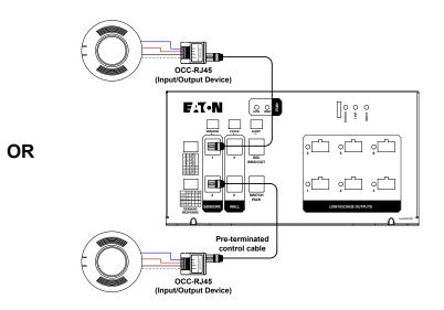
Connect the OCC-RJ45 Input/Output Device to the BMS system. Closure will be made across the Blue and Red wire locations. Connect a pre-terminated control cable between the REC/BMS/OUT RJ45 port on the Power Module and to one of the ports on the OCC-RJ45 ports.
