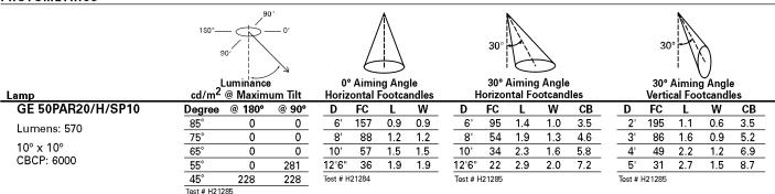
Note: Photometrics are from P3120-E3AAC, actual performance using E3PINLARGE element will be less.
