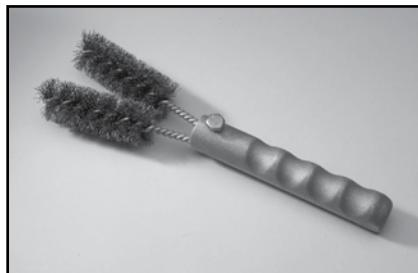
The Card Cloth Brush is used for cleaning large conductors and bus bar. It has short stiff bristles. These brushes are for cleaning cable only, not molds.
