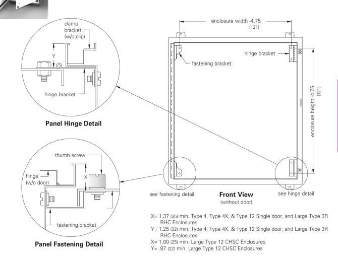
Notes: Large Type 12 CHSC Enclosures have back panels installed. Dimensions are in inches. Millimeters shown are for reference only.
