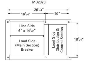
2. Use anchor bolts (<sup>3</sup>/8" dia.) pre-cast in concrete pad. Mounting hole dimensions are shown above. Locate line and load conduits the same as in method 1.
