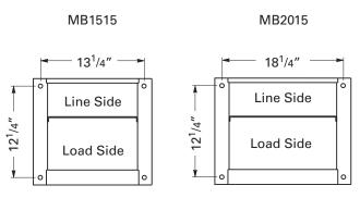
Use anchor bolts (<sup>3</sup>/8" dia.) pre-cast in concrete pad. Mounting hole dimensions are shown above for 15 x 15 and 20 x 15 pedestals. Locate line and load conduits the same as in method 1.
