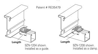
When installing this device as an expansion guide on the outside flange of Steel Side Rail, use the Catalog No. B202 Square Washer in order to properly elevate the guide.
