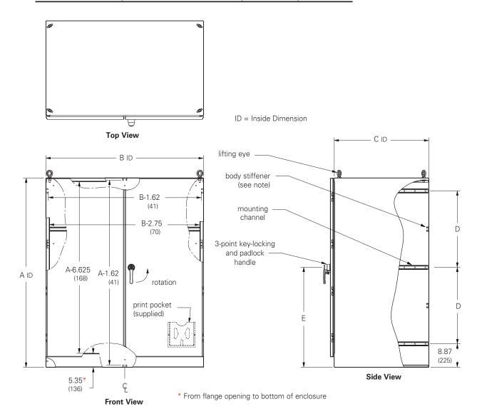
**Notes:** Two body stiffeners spaced evenly along enclosure height. Two lifting eyes are furnished when C dimension is less than 36.00 (914 mm). Dimensions are in inches. Millimeters shown are for reference only. Data subject to change without notice.
