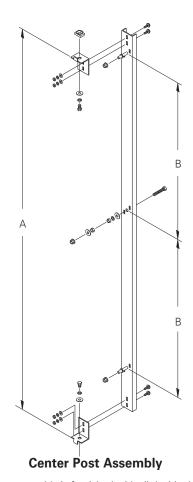
Center Post assembly is furnished with all double-door Full Panels and includes hardware necessary for channel and panel mounting. The Center Post is optional on double-door Half Panels and Swing Panel mounting and must be ordered separately. It attaches to the top and bottom channels making it adjustable along the depth of the enclosure. See illustration #5 on the Detail Sheet-page 123.
