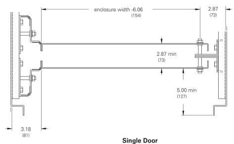
(section view showing swing panels mounted back-to-back)
