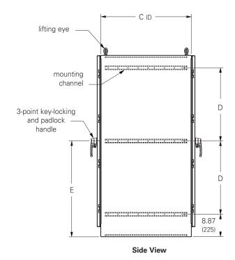
Notes: Two lifting eyes are furnished when C dimension is less than 36.00 (914 mm).
