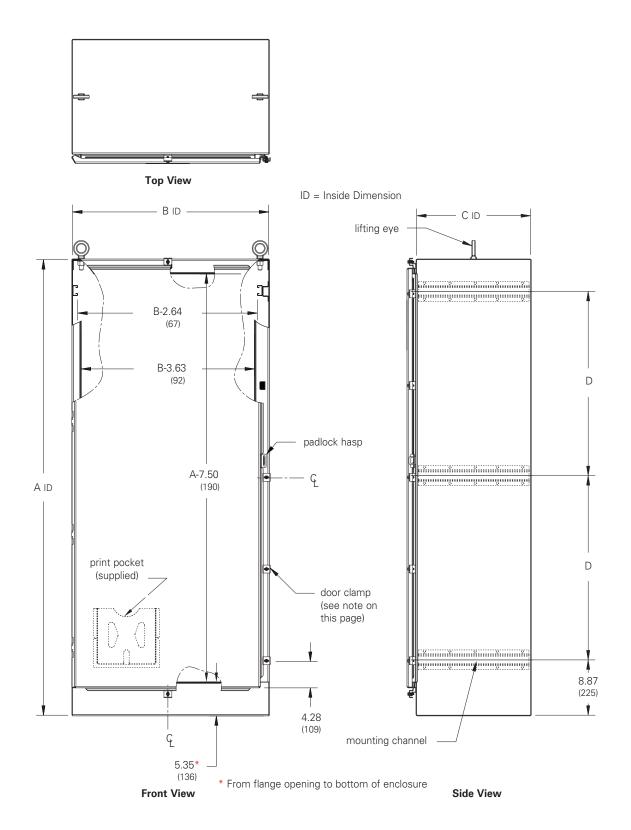
Notes: Two lifting eyes are furnished on each enclosure. Clamps are mounted along three sides of the enclosure door. Spacing between clamps along side opposite the hinge does not exceed 15 inches. Dimensions are in inches. Millimeters shown are for reference only. Data subject to change without notice.
