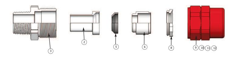
Remove and discard the resin dam (5). (This part is only needed when the connector is used with the RapidEx resin system.)
