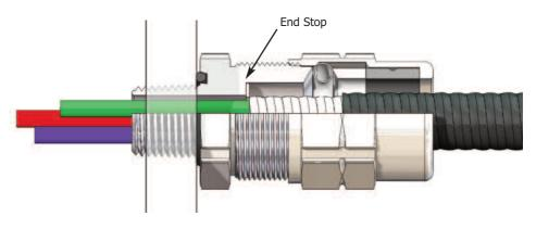
5. Finally, tighten the Outer Nut (7) to compress the Grounding Spring (4) to secure the armor, and also to compress the Jacket Seal (6) onto the cable jacket. Do not over-tighten. The Entry Component (2) and the Outer Nut (7) do not have to close face to face.
