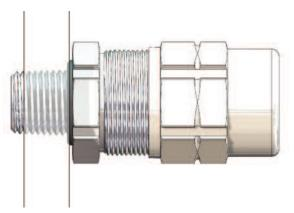
4. Pass the cable through the connector until the armor makes contact with the end stop. If it is not possible for the conductors to pass through the end stop then it should be removed so that the armor can make contact with the integral end stop within the entry component.
