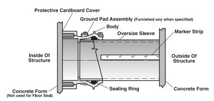
FIG. 2 INSTALLING CABLE CONDUIT OR PIPE AND SEALING ASSEMBLY
