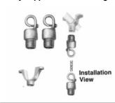
Complete assembly includes two hooks and one rigid support. Each hook supplied with a screw for closing 3/8" jaw opening. Rigid Support straddles max. 1-1/4" conduit. (Chain shown in installation view not furnished.)
