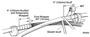
a. Insert base assemblies of shield connectors between the core wrapper and the shield 180° apart. Insert base assemblies of shield connectors between the core wrapper and the shield 180° apart. Install first nut and torque to 45 ± 5 in-lbs (5.2 ± 0.6 kg·m).
