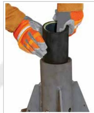
Use cylinder reducer **A2238-03** in adapter base to allow for use with 24 inch davit arms.
