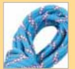
7-1/2 mm and 8 mm rope has polyester sheath and Technora core, which is fire resistant to 925°F.
