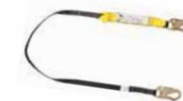
**EXTERNAL** | Tearweb is packed in a PVC sleeve and tears out during a fall arrest. External energy absorber attaches to back D-ring of harness.
